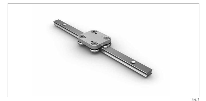
MiniRoller Rail is a steel linear guide with compact design. It has radial roller bearings that glides on an induction hardened and honed raceway. It has been developed for applications that move moderate loads within tight spaces. MiniRoller Rail also manages parallelism deviation up to 0.03 mm.
