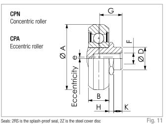
Seals: 2RS is the splash-proof seal, 2Z is the steel cover disc Note: The rollers are lubricated for life
