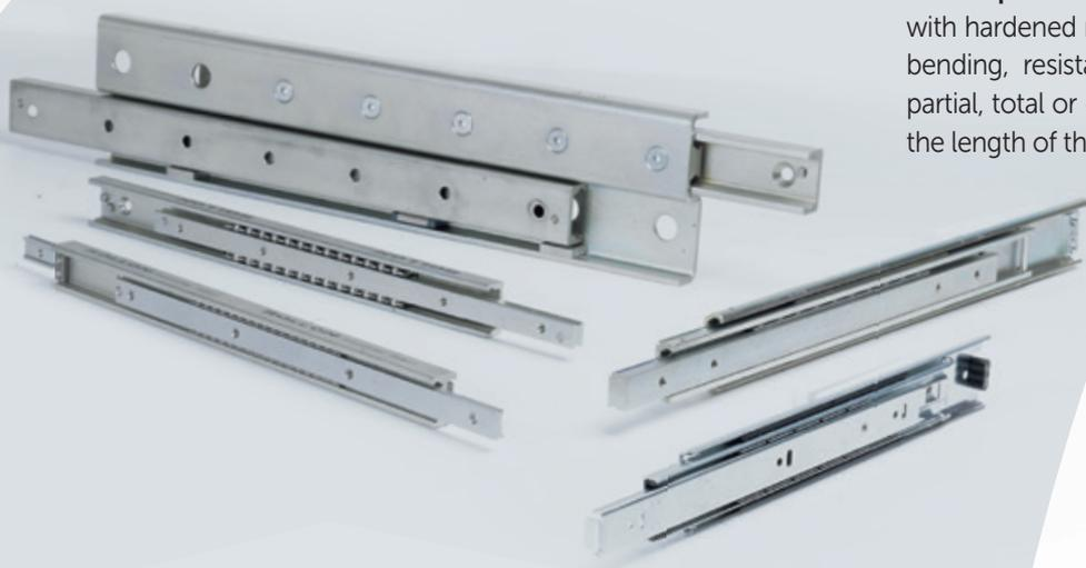
**Telescopic rails with ball and roller bearings**, with hardened raceways, high load capacities, low bending, resistant to shocks and vibrations. For partial, total or extended extraction up to 200% of the length of the guide.
