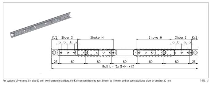
Version 2 is a variant of version 1 with several independent sliders. The total load capacity is based on the number of sliders in the rail and on their lengths. The length and stroke of the individual sliders can be different.
