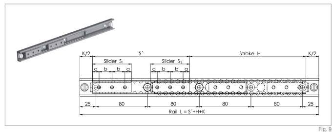
Version 3 is a variant of version 1 with several synchronized sliders. The total load capacity is based on the number of sliders in the rail. The length of the individual sliders can therefore vary. To ensure that all fixing holes of the rail are accessible, S must be < L/2 - K.
