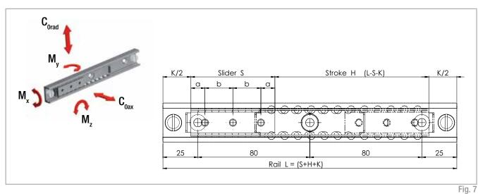
To ensure that all fixing holes of the rail are accessible, S must be < L/2 - K. To ensure proper smooth movement it is necessary that H  $\leq$  7S.
