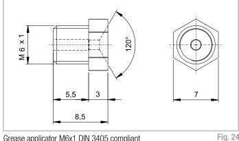
Grease applicator M6x1 DIN 3405 compliant
