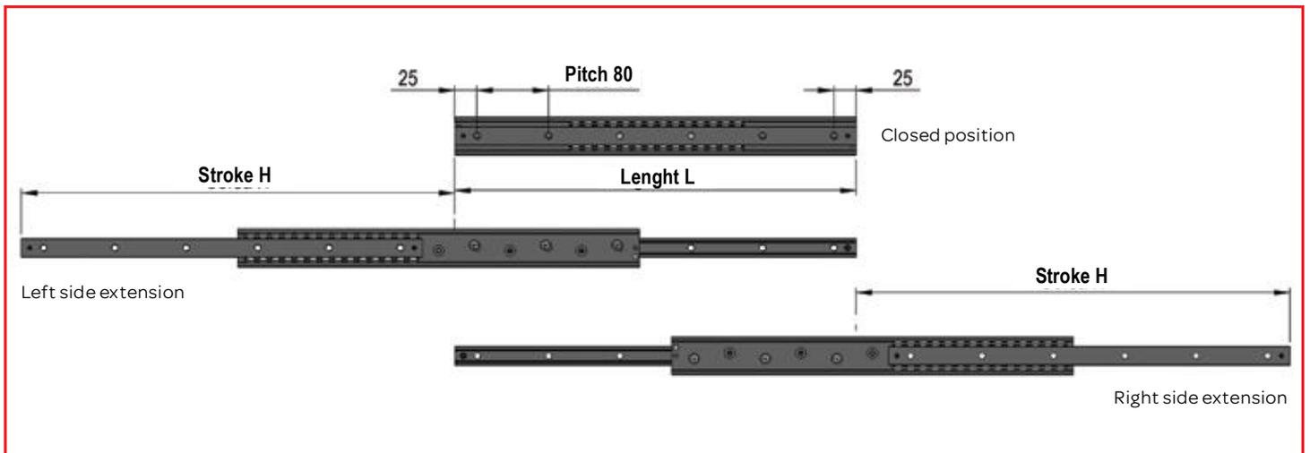
Note: The slide is provided with a set screw which limits the stroke of the movable sliders in one direction for a stroke equal to H, by removing the screw it is possible to move the sliders in the opposite direction to obtain a double stroke equal to 2H.
