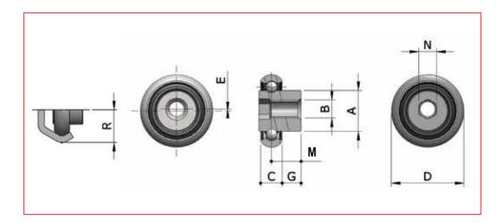
The rollers series P.. Are also available in stainless steel INOX AISI440 hardened steel for corrosive ambients.
